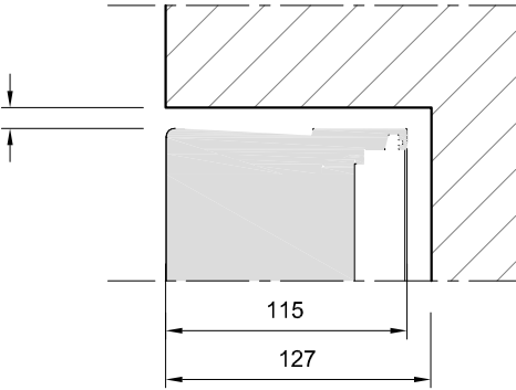
D4: recessed mounting - clearance
